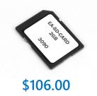
SD memory card for non-volatile storage, 2GB industrial grade. 85° C maximum operating temperature makes it suitable for data logging in industrial applications. Recommended for *C-more* EA9 series. The EA-SD-CARD utilizes SLC technology so it is the fastest option for writing and storing data. If logged data is saved to external memory, AutomationDirect recommends using an EA-SD-CARD.
