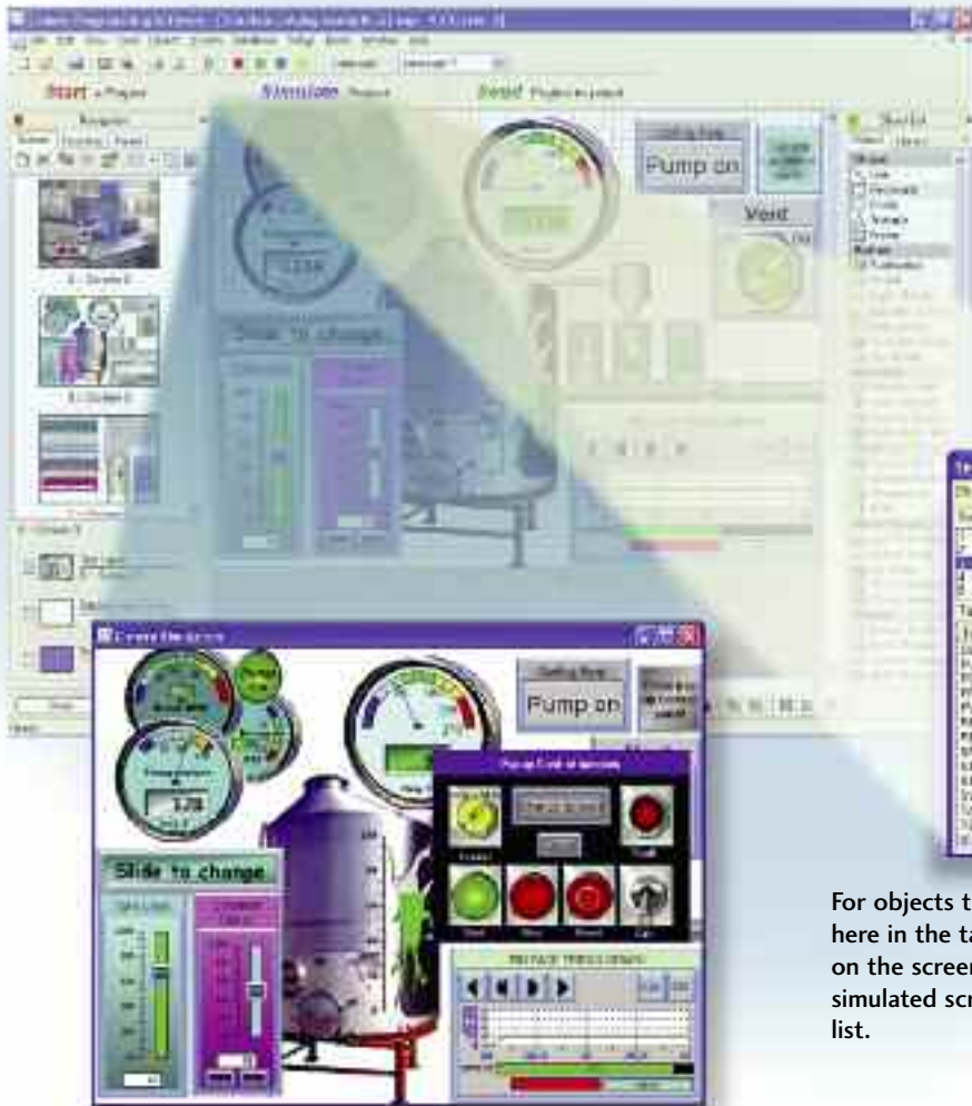
The simulation control window shows the list of screens and the tags and add their values on the highlighted screen in the list.
