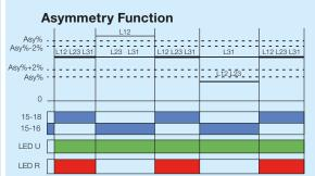
The RWM17 protector relay has state indication LEDs, as shown below:
