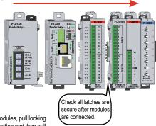
Step Two: To unstack modules, pull locking latch up into the unlocked position and then pull modules apart.
