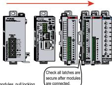
Step Two: To unstack modules, pull locking latch up into the unlocked position and then pull modules apart.
